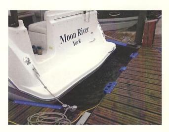
The short fender can be used as a stern/side fender or simply remove the centre membrane and this fender can be used on corners up to and over 90°. A versatile fender that is robust and easy to attach.
